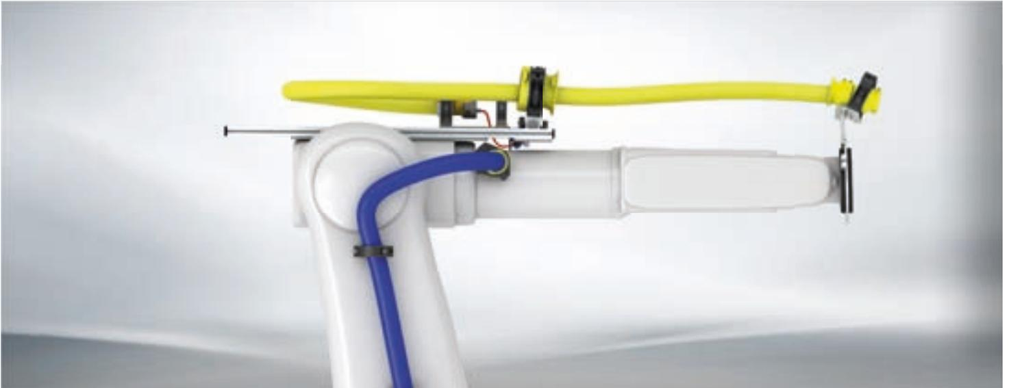
The SUMOTEX™ dresspack system uses a novel and unusual way of achieving the reset effect that is needed to be able to run the cable bundle tightly along the robotic arm, which relies on pneumatic pressure assistance integrated within a textile sheathing.
