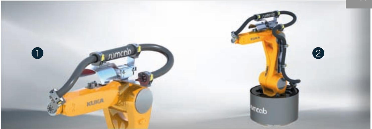
1 Dresspack system axis 3-6 suitable for corrugated hose diameters of NW17, 29, 36 Including the robot-side interface at axis 4
