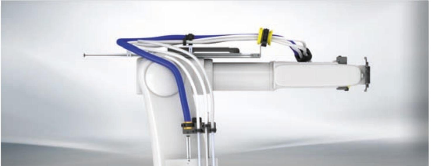
The SUMOSLIDE features an extremely compact design and a linear forward and backward movement of the spring carriage. These design features prevent tight bending radii and looping on the robot. This makes the SUMOSLIDE ideally suited for guiding corrugated tubeless components such as suction hoses, feed hoses or heating hoses.
