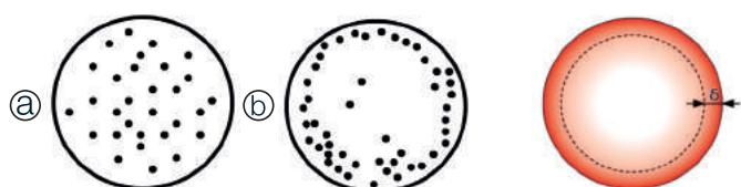
Transverse section of the current flow distribution in a cylindrical conductor. For alternate current, most of the electrical current (63%) flows between the outer surface and skin depth, , depending on the frequency of the current and the electric and magnetic properties of the conductor.
